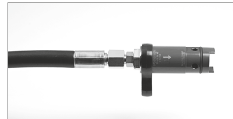
To vent, firstly isolate the pressurised fill line. Then vent the fill line by using the vent valve until the safety break on the dispenser side (the body) is without pressure.
