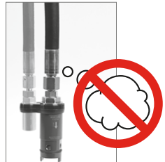
The gas flow within the fill line (dispenser side) will stop automatically when the safety break is separated. Venting must be performed afterwards.
